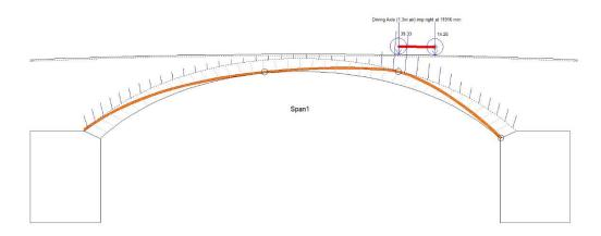
Adding a modest amount of backing makes the bridge more than adequately safe.
