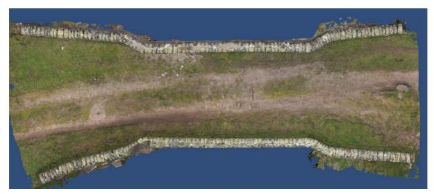
I nearly forgot to include a plan view (above). Notice the unusual plan shape of the wingwalls, with a sharp initial flare than a more gradual widening. To encourage recalcitrant cattle into the gap?
