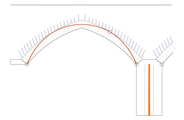
Modelling this bridge in Archie can be accomplished using the "pointed" arch shape and juggling with input data to get a sensible shape. The spandrels are likely to have been filled
