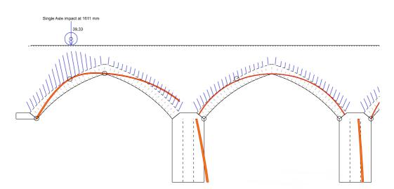
Loading with a single modern axle and balancing the thrusts as best I can shows the bridge rather weak without any backing. In this form, the left hand span would probably collapse as a result of tilting rthaer than collapse of the pier.
