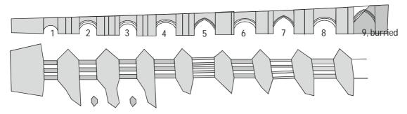
This elevation of the remains of the bridge is traced from a drawing by Stewart Brown. There were originally 17 or 18 spans. The 9th now vanishes under a new road. The sketch plan above shows how the builders dealt with a skew flow using spans skewed at up to10 degrees and cutwaters further skewed to meet the flow.
