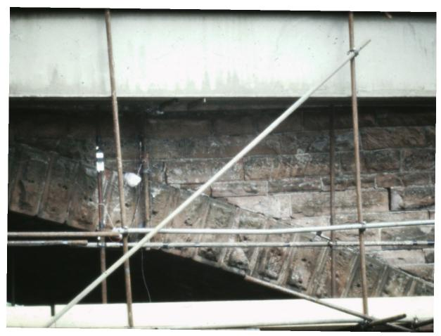
Here we see the same area rather later in the test. The joint between arch and spandrel is visibly damaged over a long length. The voussoirs are about 300mm thick so the picture shows 4m length of arch. The loaded 1/4 span point is behind the scaffold tube with the white tab attached.
