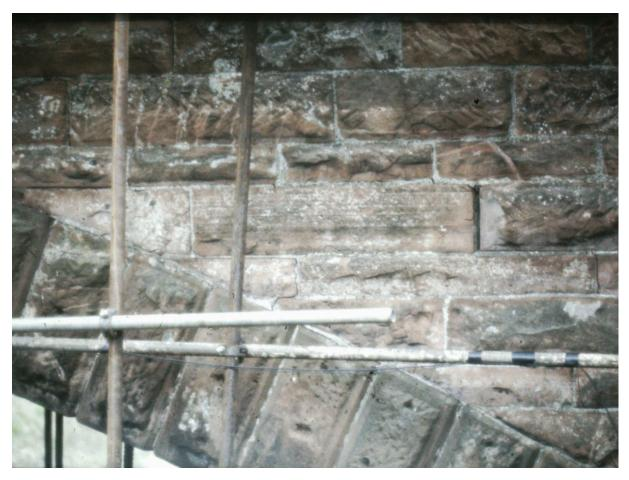
This enlarged image Shows an area of spandrel and arch directly under the load at an early stage in the test. Look carefully and you will see cracks between the two voussoirs to the left, which are nearest t the load point. In the top right there is a horizontal crack between two stones indicating a corbelling of the spandrel wall.
